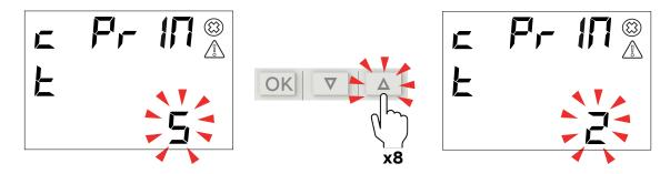
If during the data entry the desired number is exceeded by mistake, it is needed to increase the displayed number until data entry starts again from 0.
