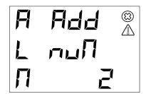
• "Add" indicates that the alarm is not yet present. If it needs to be added, press the button "**OK**" to go to the event and configure the subsequent parameters.
