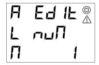
"Edit" indicates that the alarm is already present. If it needs to be modified, press the button "OK" to go to the event and modify the configurations.
