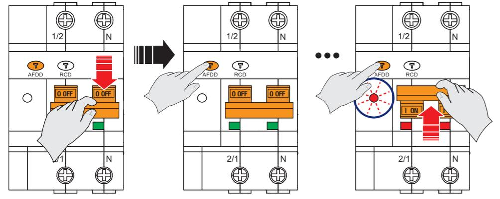
**Clearing of the memory of the last LED indication due to arc fault tripping or overvoltage**
