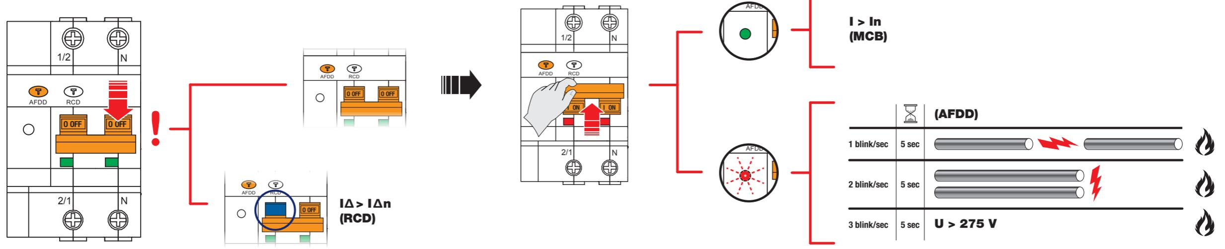
**Recall of the last LED indication due to arc fault tripping or overvoltage**
